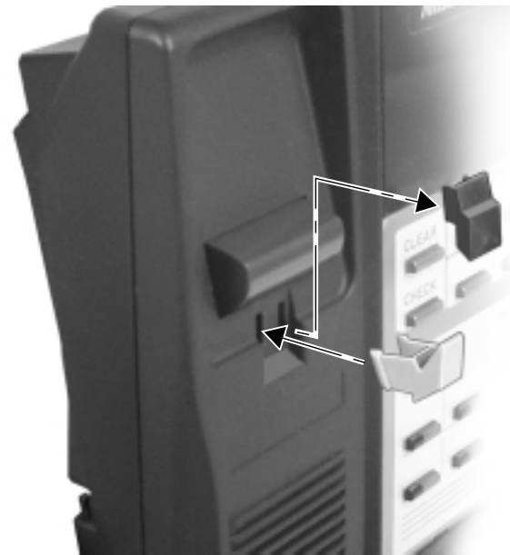
Figure 4-10 INSTALLING THE WALL-MOUNT HANGER
