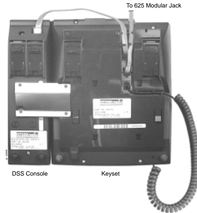
Figure 4-7 INSTALLING A 24-BUTTON DSS CONSOLE 4-15
